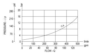
Measured with hydraulic fluid ISO-VG46 at 36° ±2 °C (97° ±36 °F); ambient temperature 23 °C (73 °F).
